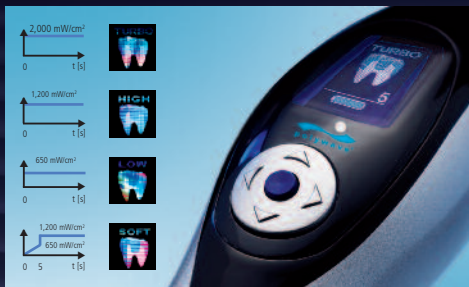
Four easy-to-use programs – Turbo for maximum performance, High Power for rapid curing, Low Power for curing areas near the pulp and Soft Start for stress-reduced polymerization.
