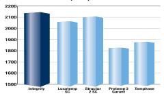
Flexural Modulus measures the degree of bend in a material prior to fracturing. A material with a low flexural modulus can create undue stress in the cervical region. This subjects the temporary cement to shear compression and tensile forces that can weaken the bond. Generally, the higher the flexural modulus number, the stronger the bond.
