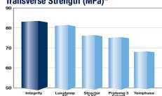
Transverse Strength is a strength test of a beam of material, supported at each end, and placed under a load. Higher numbers are preferable, with 80 MPa being the minimum acceptable ISO standards measurement. A higher flexural strength is a good measure of resistance to marginal fracture.
